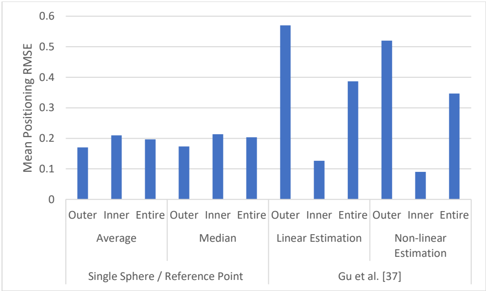
Figure 5.2: Illustration of the mean positioning RMSE of the single sphere per reference point and the method proposed by Gu et al. [41].
