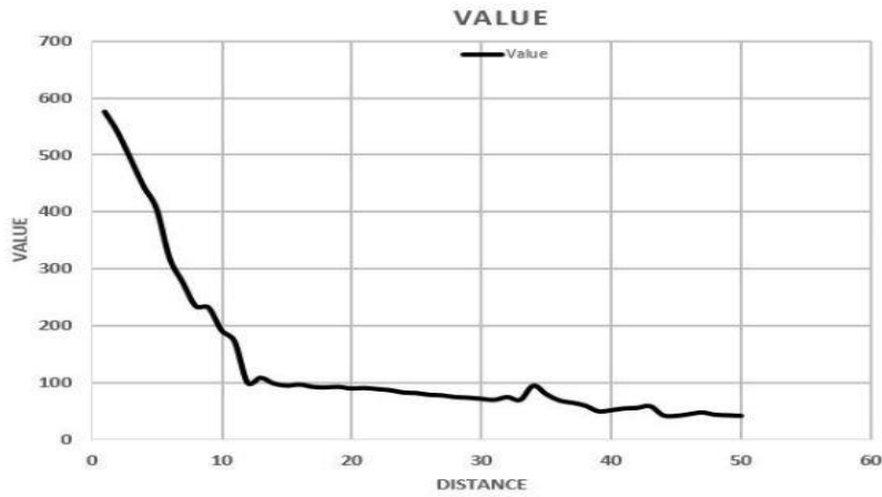
Figure 2.5: Flame sensor value vs distance.
