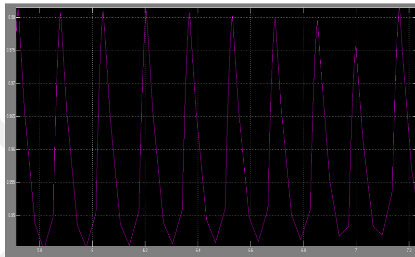
Figure 5.8: The steady state error for proportional derivative controller by using fuzzy logic control with DC Motor system by scope in MATLAB.
