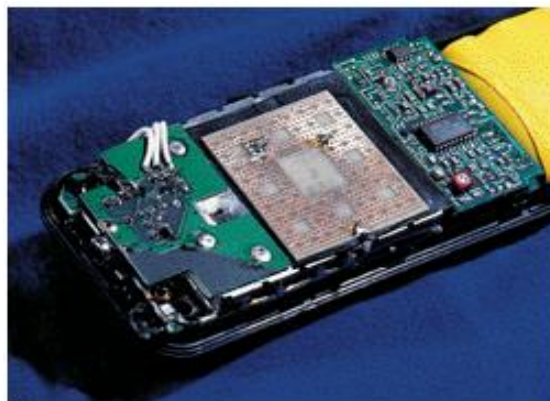
Figure 1.1: A photo of the Sierpinski carpet used to fabricate an internal antenna of a mobile phone covering the 900 MHz, 1800 MHz, and 1900 MHz bands [2].
