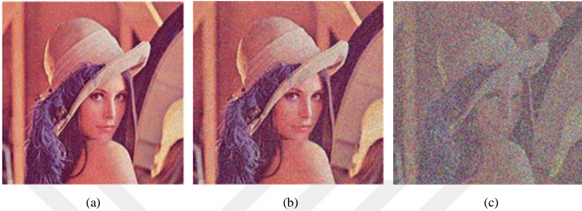
Figure 5.5: Recovered images after salt and pepper noise is added: (a) salt and ppepper with density 0.05, (b) salt and ppepper with density 0.1, (c) salt and pepper with density 0.5.
