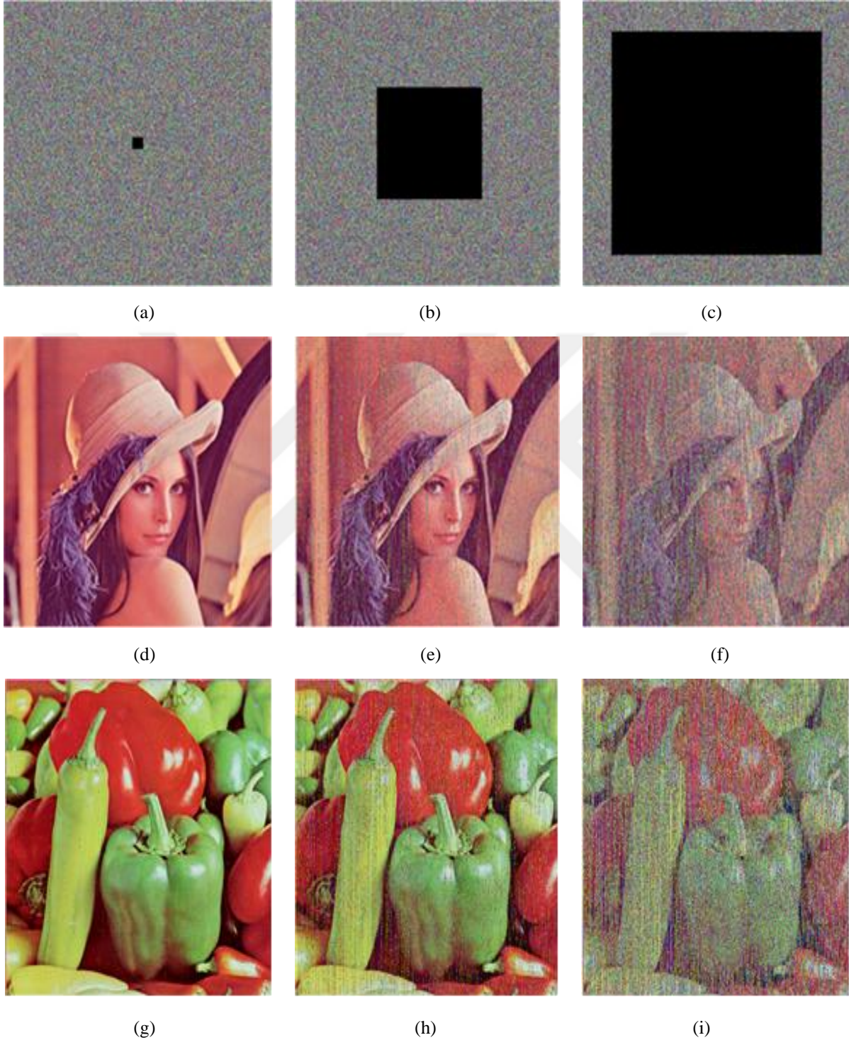
Figure 5.7: Data lose attacks test: (a) encrypted image with data lose ( 20 \times 20 ), (b) encrypted image with data lose ( 200 \times 200 ), (c) encrypted image with data lose ( 400 \times 400 ), (d) recovered image of (a) by algorithm 1, (e) recovered image of (b) by algorithm 1, (f) recovered image of (c) by algorithm1, (g) recovered image of (a) by algorithm 2, (h) recovered image of (b) by algorithm 2, (i) recovered image of (c) by algorithm2.
