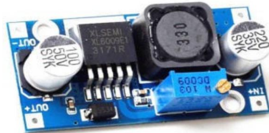
Figure.2.22: Arduino Boost Converter XL6009.
