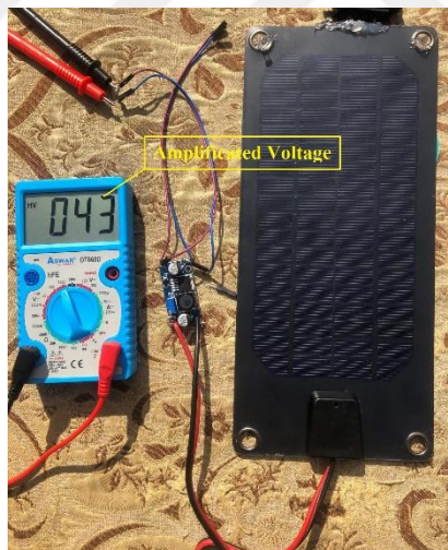
Figure 3.5: The Amplificated Voltage of Solar Cell.
