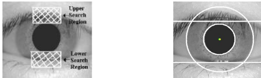
Figure 1.13: (a) Upper and Lower Search Regions of the Iris Image. (b) Upper and Lower Eyelids Detection
