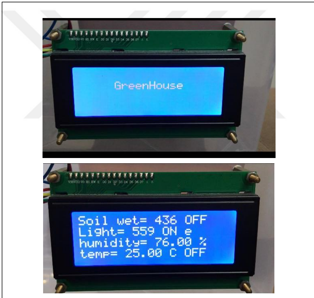
Figure 5.1: LCD Screen Showing the Sensors Data and Devices States.
