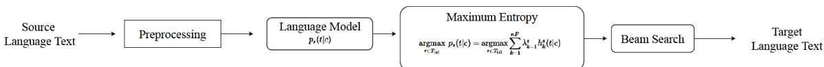
Figure 4.3: Architecture of the translation approach based on maximum entropy models. In addition, the maximum entropy approach has various benefits such as we can easily extend by adding more features, and it is possible to incorporate into different SMT models
