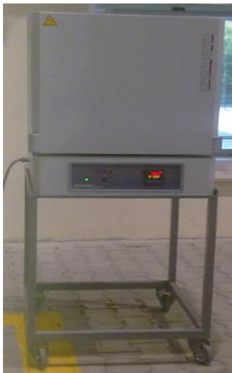
Figure 3.3: Pictures of Furnace
