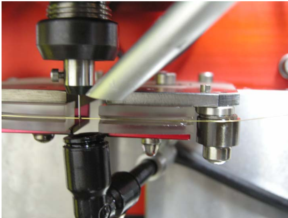
Figure 3.5 Electrode dressing by wire dressing unit
