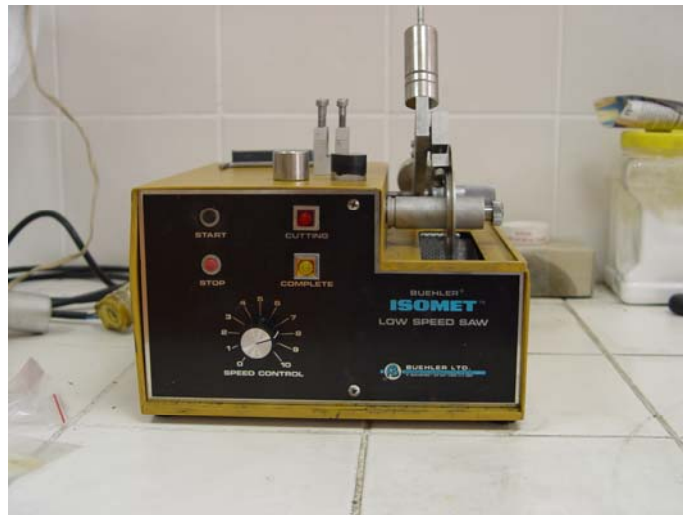
Figure 3.11 Buehler precision isomet low speed saw
