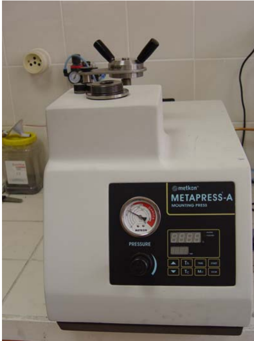
Figure 3.12 Automatic hot mounting press
