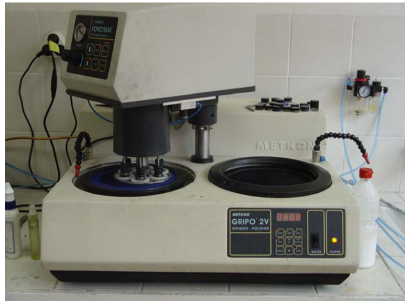
Figure 3.13 Grinding and polishing machine
