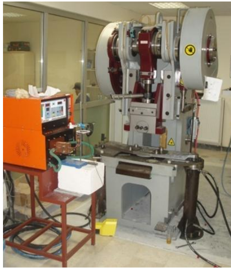
Figure 5.10: C type mechanical press.
