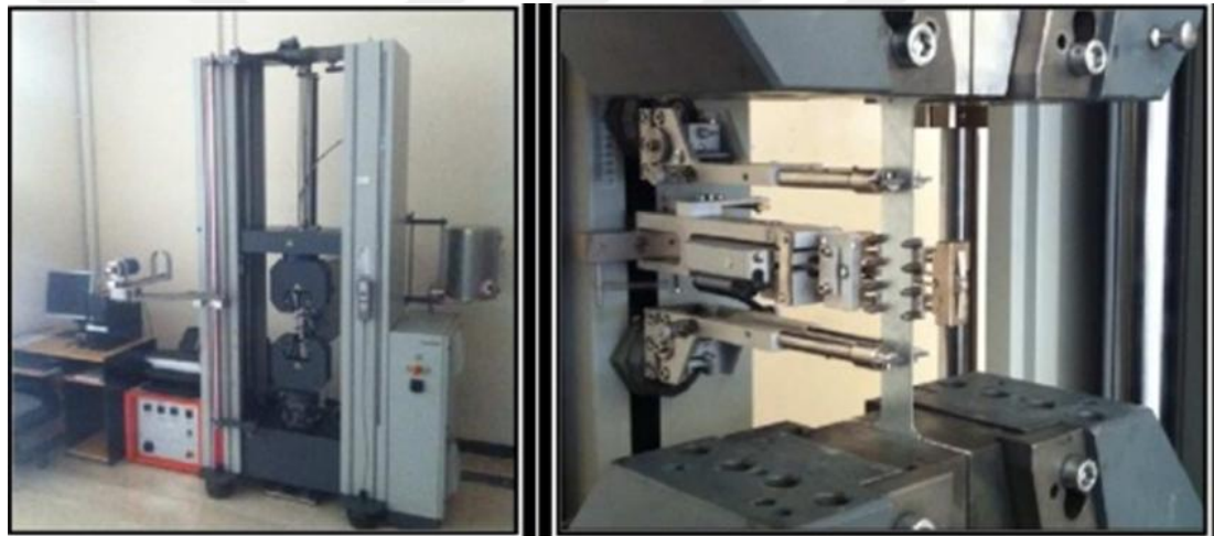
Figure 5.3: Zwick Roell Z300 Tension/Compression Test Device
