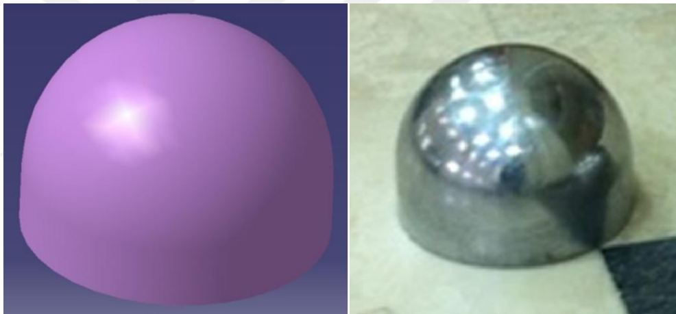
Figure 5.23: General view of the hemispherical punch.
