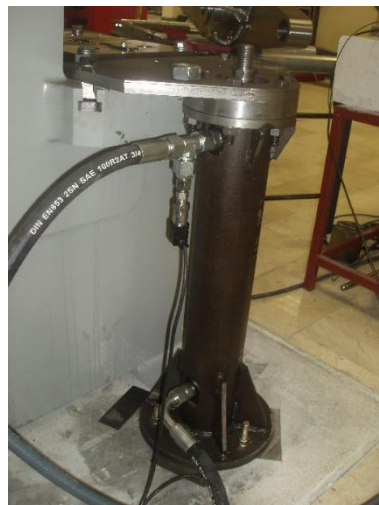
Figure 5.15: Pressure transducer attached on hydraulic cylinder.
