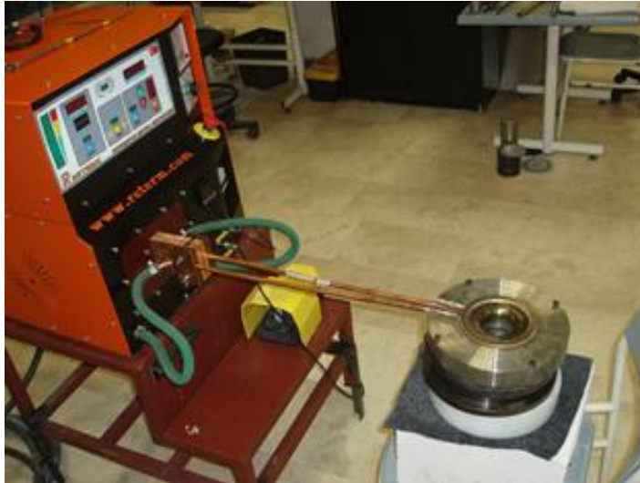
Figure 5.12: Induction heating system.
