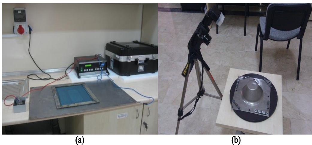
Figure 4.36 GOM-Argus optical forming analysis system in MFCE, (a) the etching system with stencil and marker head, (b) camera system and coded reference points .
