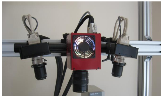
Figure 3.8 Aramis system with CCD cameras and a light source.
