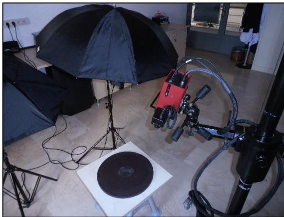
Figure 4.29 The GOM-Atos 3D coordinate measurement system.
