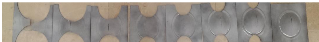
Figure 3.17 Deformed Nakazima test geometries.
