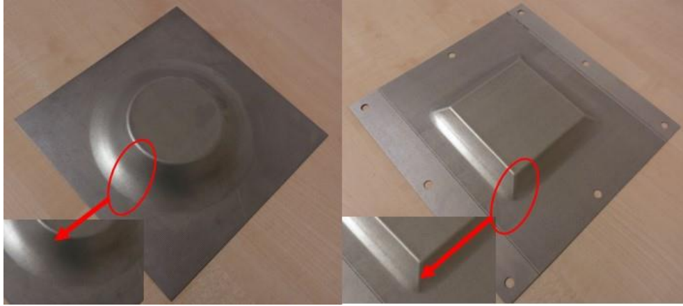
Figure 2.2 The deformation behaviors are different at lateral sides and transition regions.
