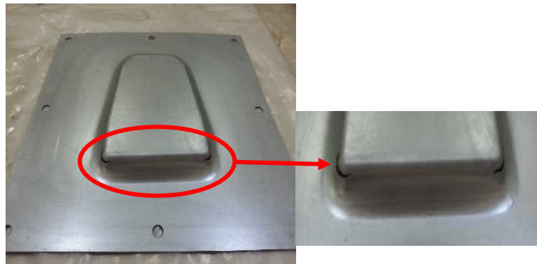
Figure 4.4 Manufactured real car component with tear.
