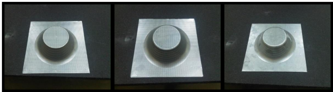
Figure 4.9 The formed parts in which 5 mm, 10 mm and 15 mm tools are used illustrated from left to right.
