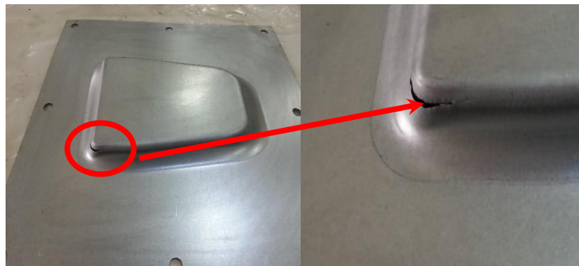
Figure 4.17 Due to high localized deformation the blank is torn.
