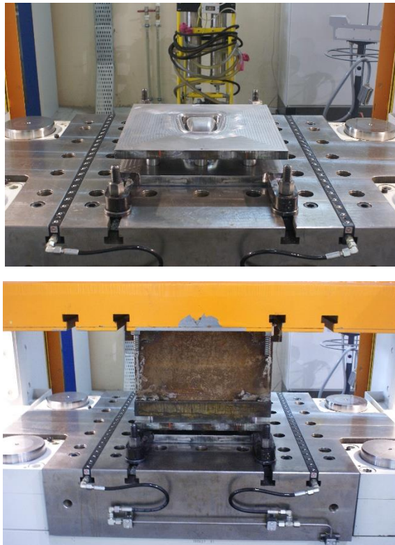
Figure 5.37 The die setup for deep drawing of the real car component.
