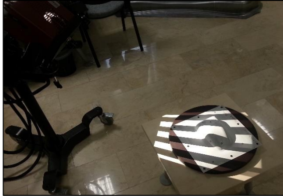
Figure 4.30 The system is based on triangulation system.
