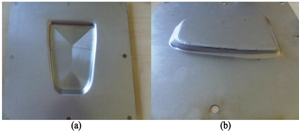
Figure 4.21 (a) is the bottom view of failed part and (b) is the top view.
