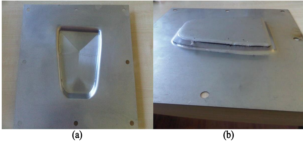
Figure 4.20 (a) is the view from bottom base of failed part and (b) is the view from top base.
