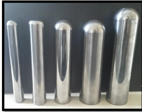
Figure 4.2 The different diameter of the spherical tool tips which are used for manufacturing the parts in a general ISF process.
