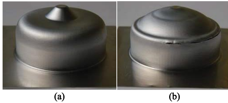
Figure 4.3 (a) The manufactured part with the achievement of D-D-D-U strategy and (b) is the failed part [56].
