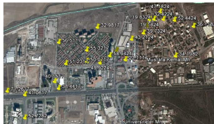
Figure 4.7 - Conversion results of the measurement values dBμV/m to dBm unit
