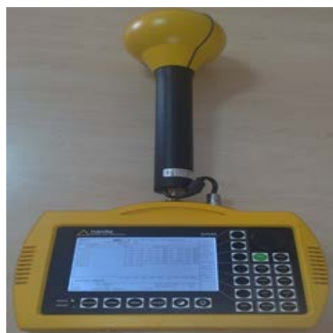
Figure 3.1 - Narda SRM 3000 and its isotropic 100 KHz to 3 GHz probe
