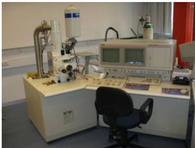
Figure 3.2. (a) Simple schematic representation of scanning electron microscope [43] and (b) used SEM device
