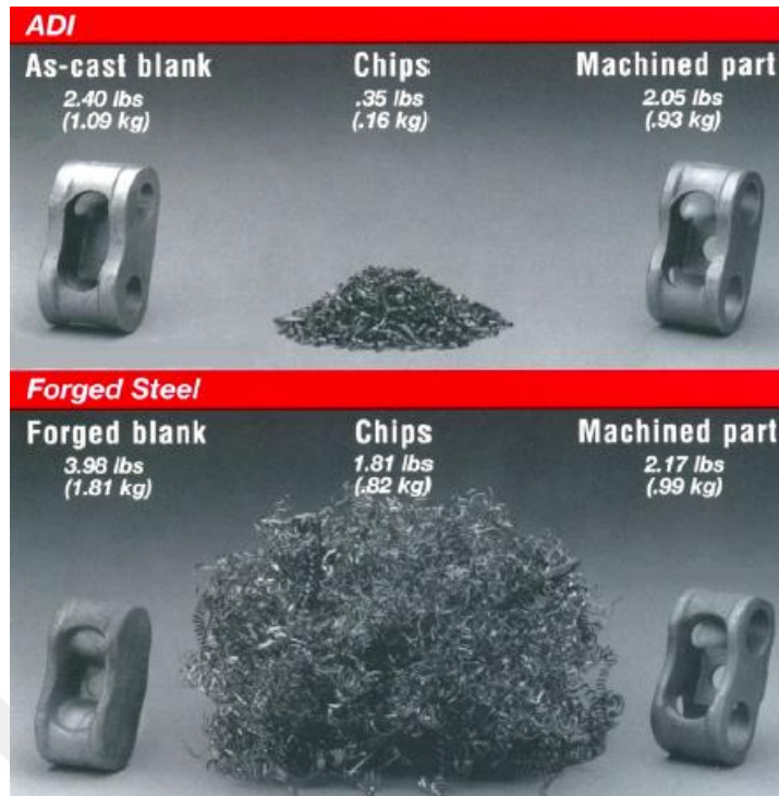
Figure 2.7-5 Cast ADI end connectors compared to forged steel in a manufacturing sequence [63]
