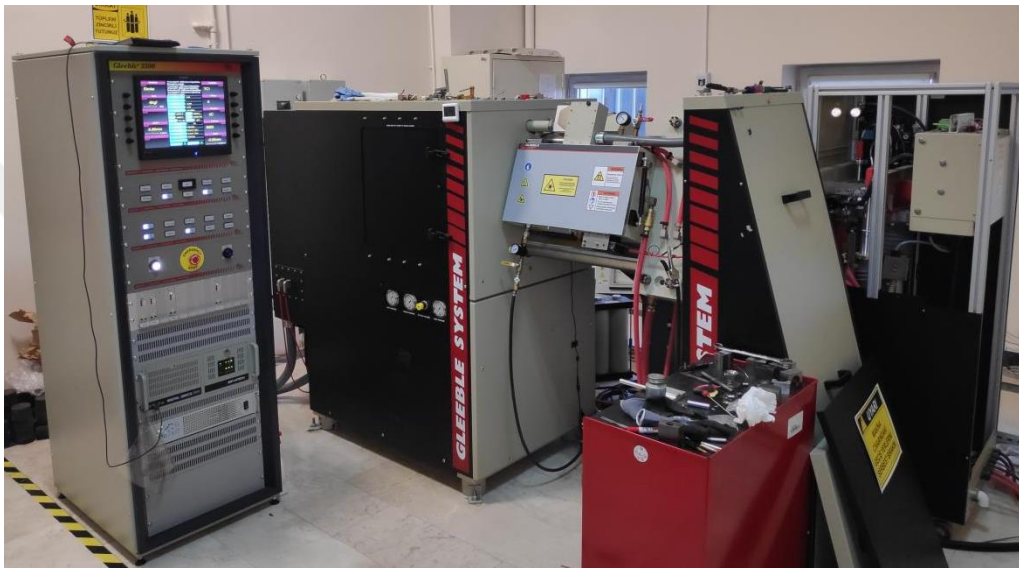
Figure 3.2-1 The Gleeble 3500 System used for this study
