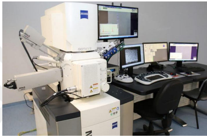
Figure 3.3-2 Carl Zeiss: Merlin – Field Emission Scanning Electron Microscope
