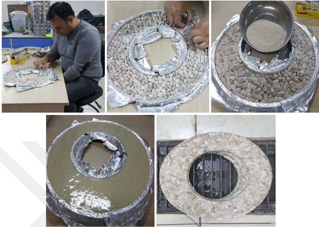
Figure 3.9 Photos from production process of the chip seal samples
