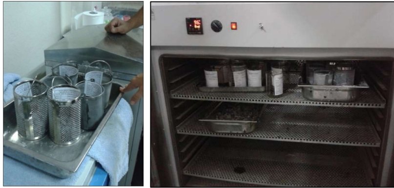
Figure 3.3 Thermal weathering resistance test
