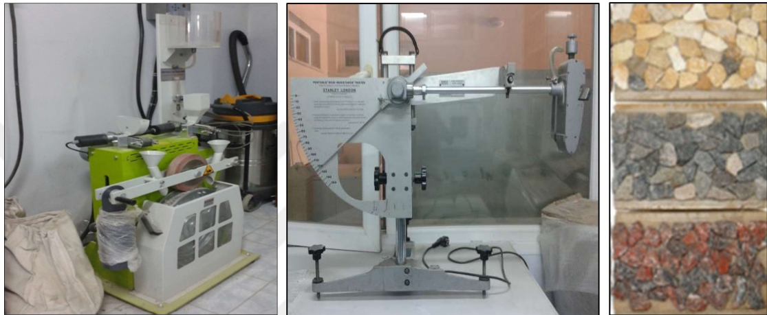
Figure 3.4 Polising resistance test aparatus and samples
