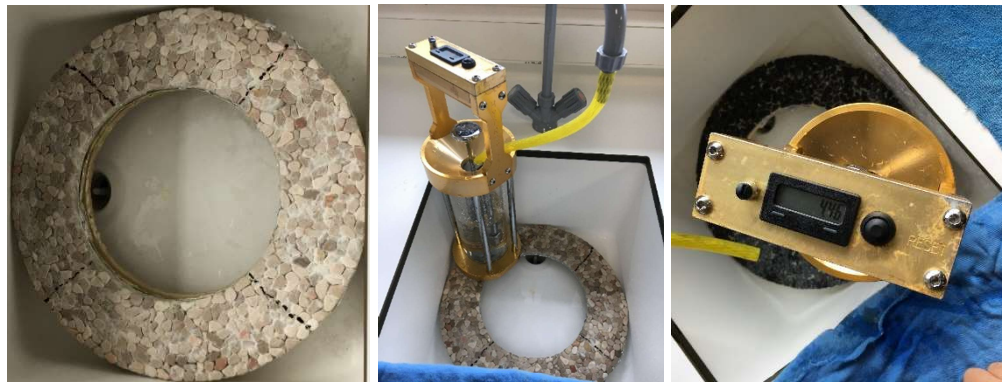
Figure 3.10 Test operation with Hydrotimer
