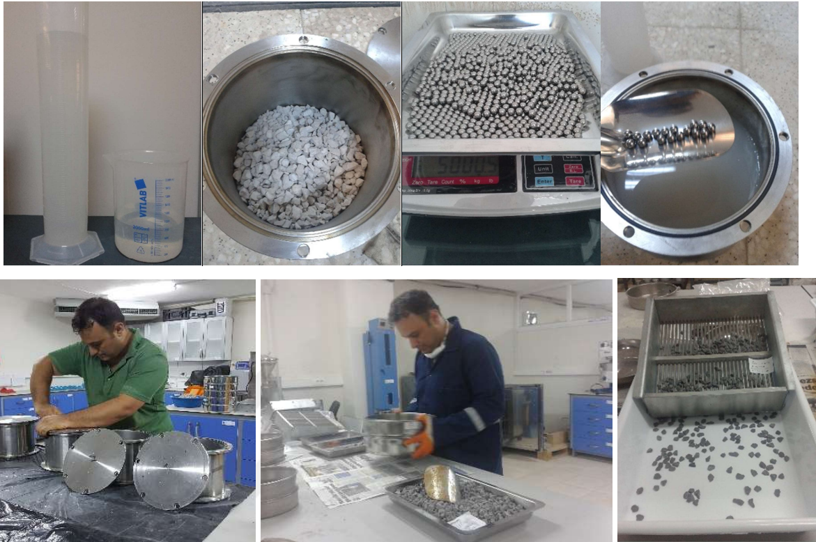
Figure 3.7 Polishing process steps with MD apparatus
