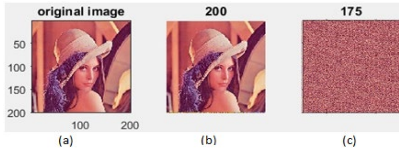
Figure 4.3 Encryption process a) original image; b) image at full period; c) Encrypted image at iteration 175.
