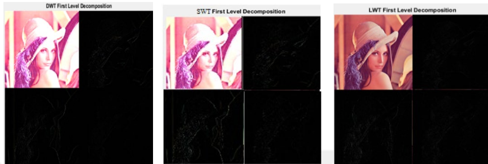
Figure 4.26 Comparison between DWT, SWT and LWT Decompositions
