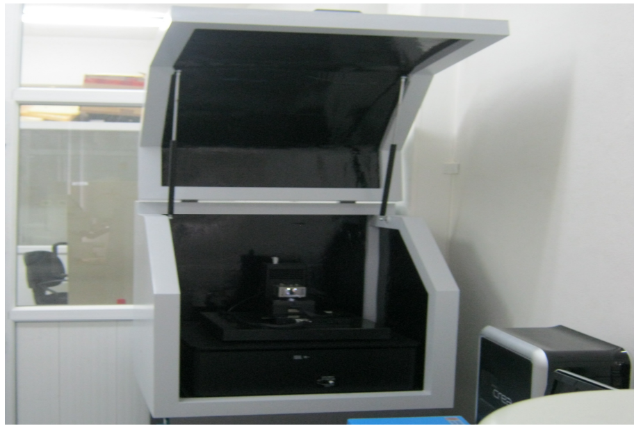
Figure 3. 16: Atomic force microscopy, AFM, (Nanomagnetic Instrument)
