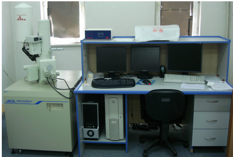
Figure 3. 11: JEOL JSM-6390LV Scanning Electron Microscope
