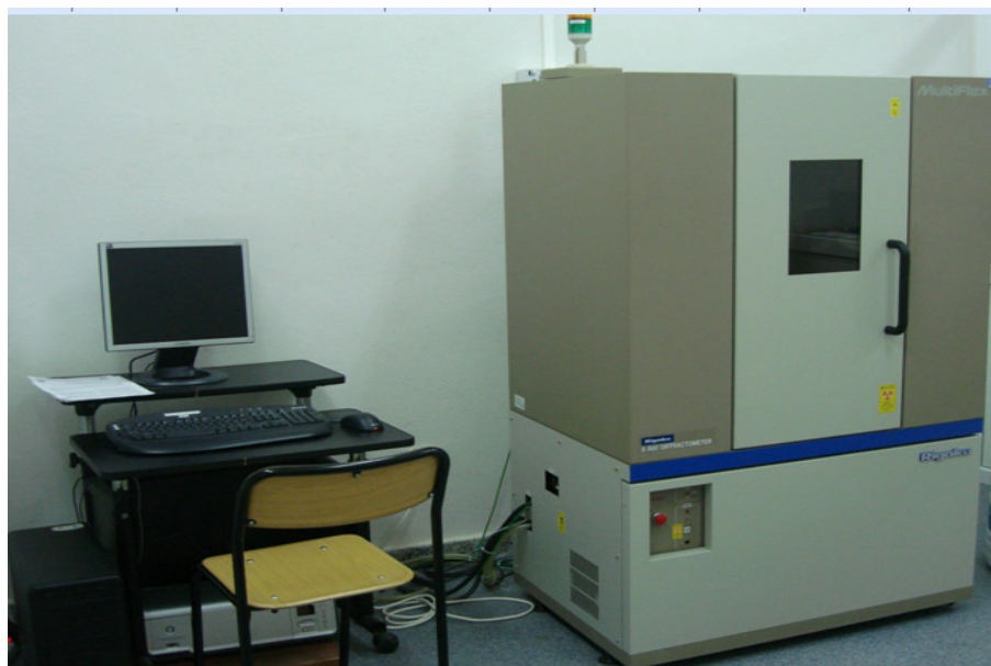
Figure 3. 13: Rigaku MultiFlex 2kW X-Ray Diffractometer
