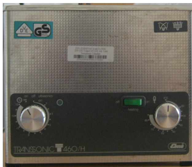
Figure 3. 6: Trassonic 460/H ultrasonic cleaning unit
