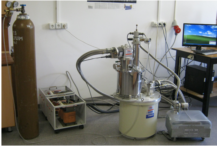
Figure 3. 14: Cryostat system for the resistivity measurements
