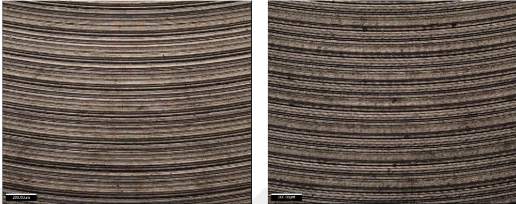
Figure 4.40 Optical Microscope Images of Finish Cut, Wet Condition, Without (Left) With (Right) Ultrasonic Vibration (78.5 m/min, 0.05 mm/tooth)
