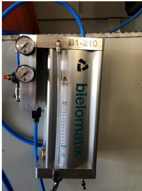
Figure 3.6 Oil tank of the MQL system
