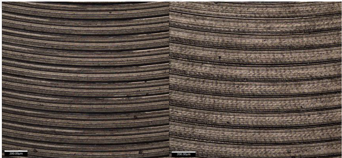
Figure 4.39 Optical Microscope Images of Rough Cut, Dry Condition, Without (Left) With (Right) Ultrasonic Vibration (78.5 m/min, 0.05 mm/tooth)
