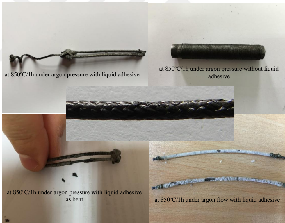
Figure 5.16. Images of the isolated wires after sintering under different conditions.
