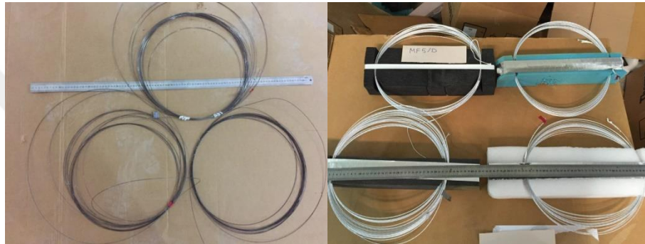
Figure 5.11. Images of the fabricated long MgB 2 /Fe wires before (a) and after (b) S-Glass braiding.
