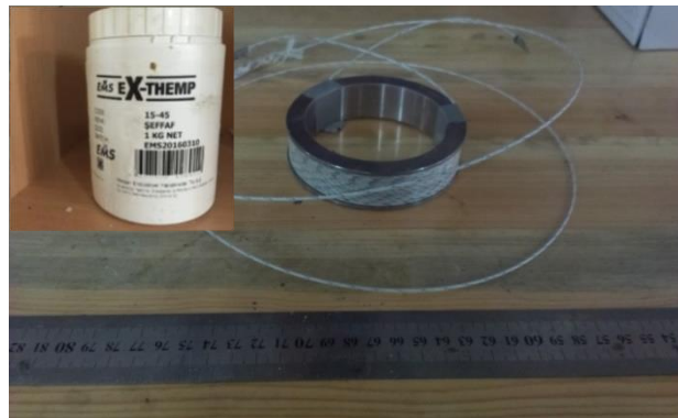
Figure 5.14. Image of the solenoid coil wound on a steel former and coated with EX-THEMP glue before heat treatment.
