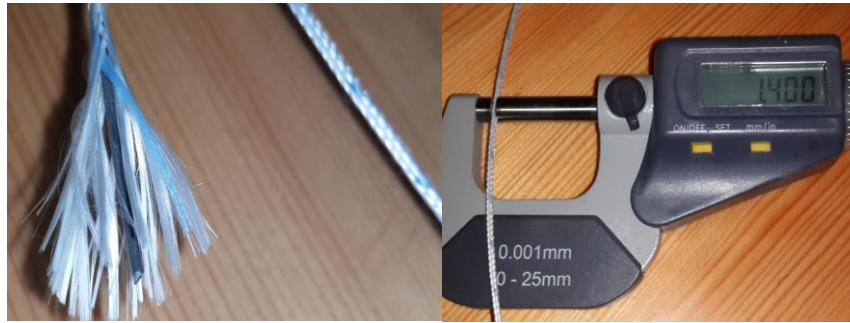
Figure 5.13. Image of the produced wire 1.10 mm in diameter after braiding with S-glass fiber
