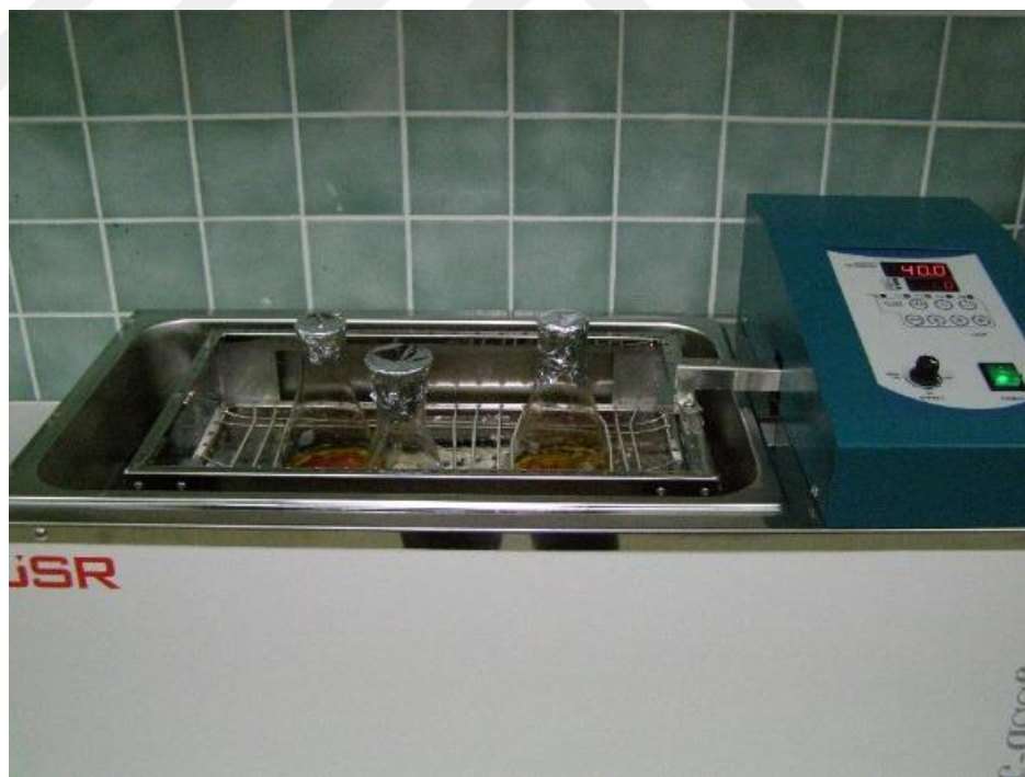
Figure 3.4. Extraction with hot shaking water bath
