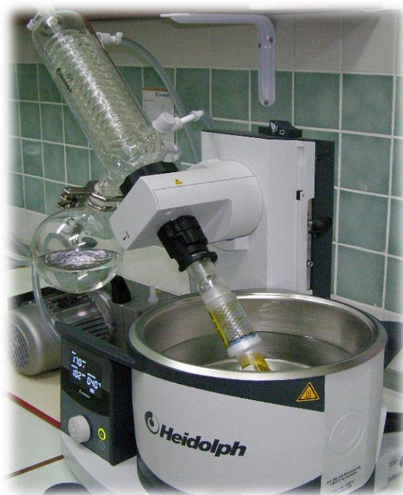
Figure 3.7. Evaporation of extraction solvent with rotary evaporator
