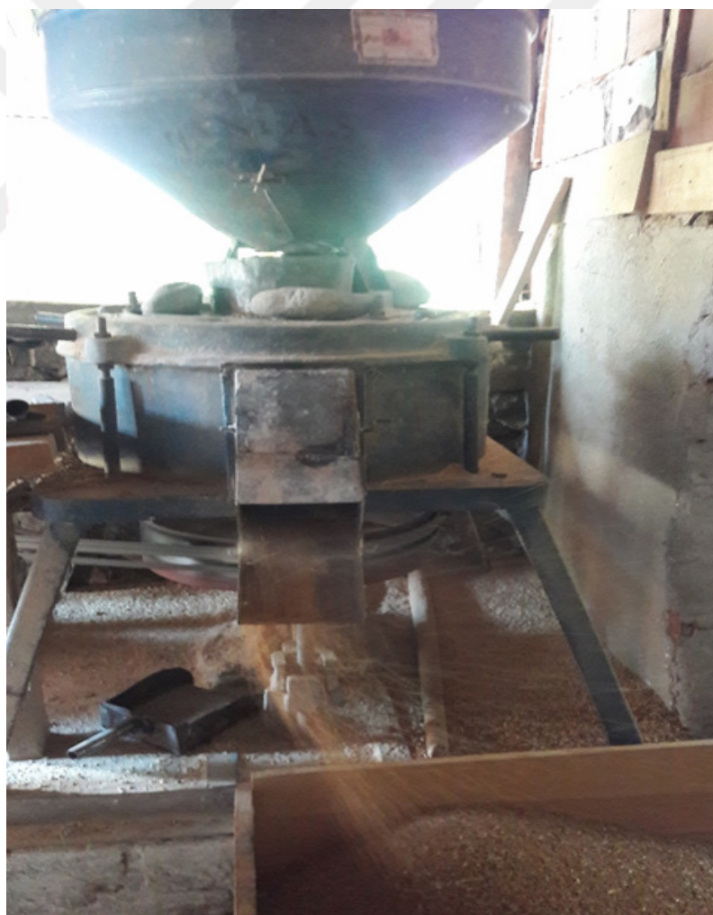
Figure 3.4 Separation of milled einkorn, by electrical stone mill, into parts of chaffs and dehulled and broken grains in Kastamonu, İhsangazi (Photo by HM Yaman)
