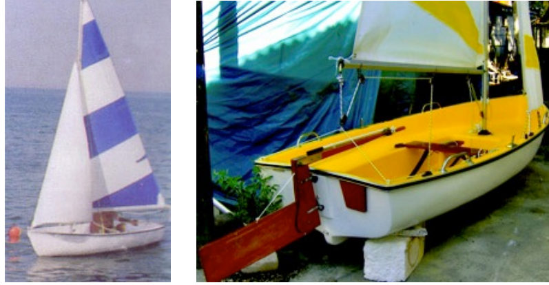
Fig. 2.3 a/b Modern Kırlangiç type boat with and without the sail and a detail of the rudder which Hammer claims resembles the tail of a sparrow.
