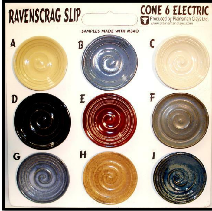
Fotoğraf 70: Plainsman Clays'in Ravenscrag Sırları, 1200°C, Numune Panosu Kaynak: http://digitalfire.com/4sight/education/ravenscrag_slip_is_born_332.html
