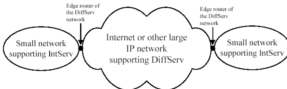
Figure 4.1 Example of an Intserv over DiffServ network.
