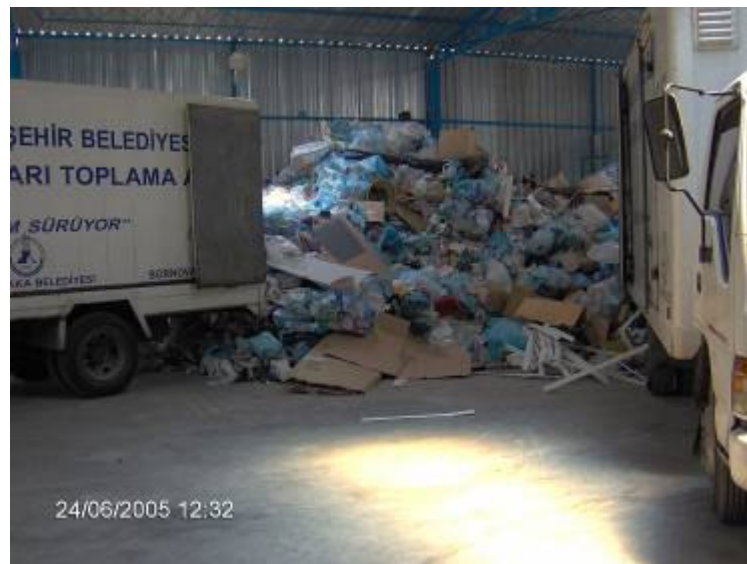
Figure 8.15 The picture of the Sorting Facility in Uzundere Compost Factory, the storage area for commingled recyclable materials before they are sorted
