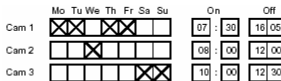
Figure A.17 Diagram explaining weekly timer
