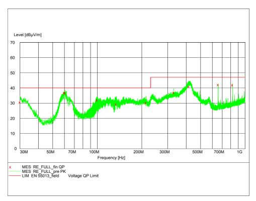
Figure 4.4 Radiated Emission test scan result of a TFT LCD TV in Semi Anechoic Chamber
