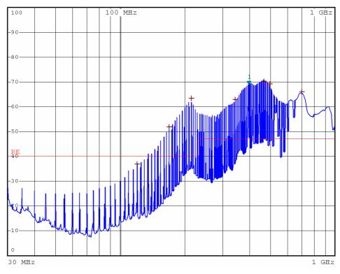
Figure 4.8 Radiated Emission test scan result of a Field Reference Source for vertical polarization of the antenna in Full Anechoic Chamber
