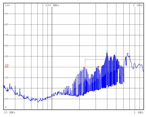
Figure 4.7 Radiated Emission test scan result of a Field Reference Source for horizontal polarization of the antenna in Full Anechoic Chamber
