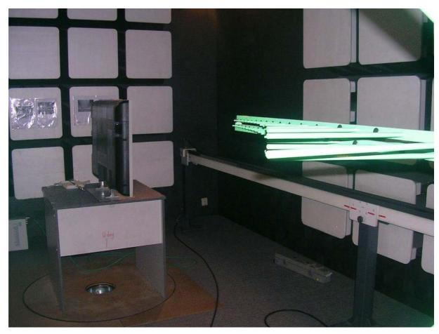
Figure 4.1 Measurement setup of a TFT LCD TV in Full Anechoic Chamber
