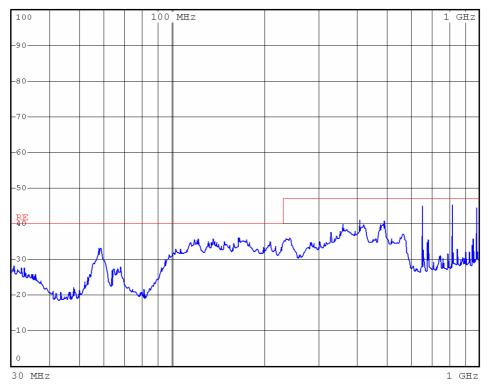
Figure 4.2 Radiated Emission test scan result of a TFT LCD TV in Full Anechoic Chamber
