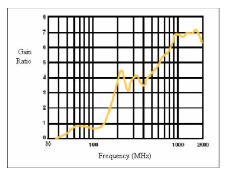
Figure 3.27 CBL 6112 gain ratio
