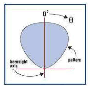
Figure 3.8 Polar plot of the response of tha antenna
