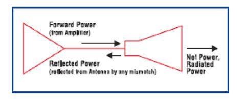
Figure 3.12 Power terms of the antenna
