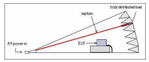
Figure 3.33 The GTEM cell – side view
