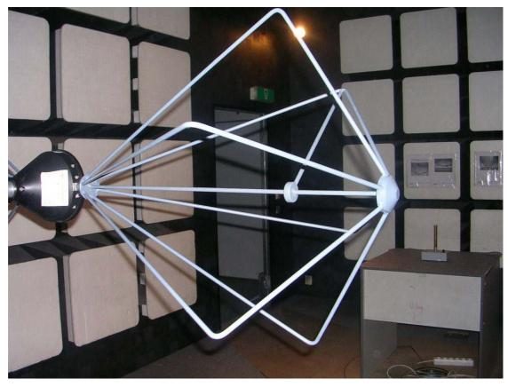
Figure 4.6 Measurement setup of a Field Reference Source in Full Anechoic Chamber
