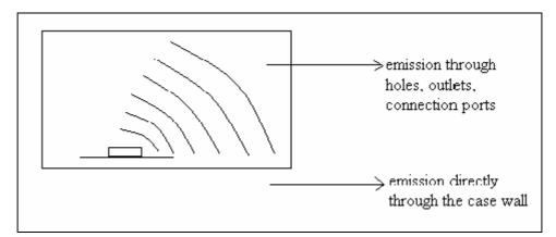
Figure 3.2 Transmission from inside to outside
