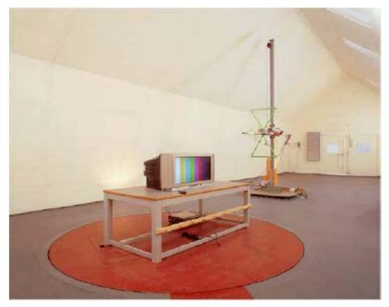
Figure 3.35 Covered Open Area Test Site
