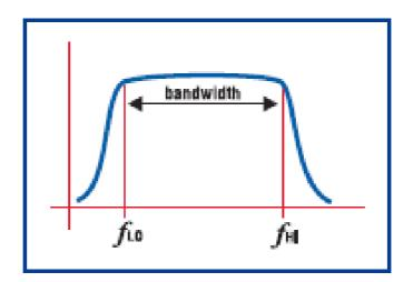
Figure 3.11 Bandwidth of the antenna
