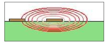
Figure 2.4 Inductively coupled (magnetic field)
