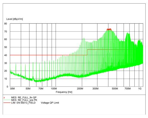
Figure 4.11 Radiated Emission test scan result of a Field Reference Source for vertical polarization of the antenna in Semi Anechoic Chamber
