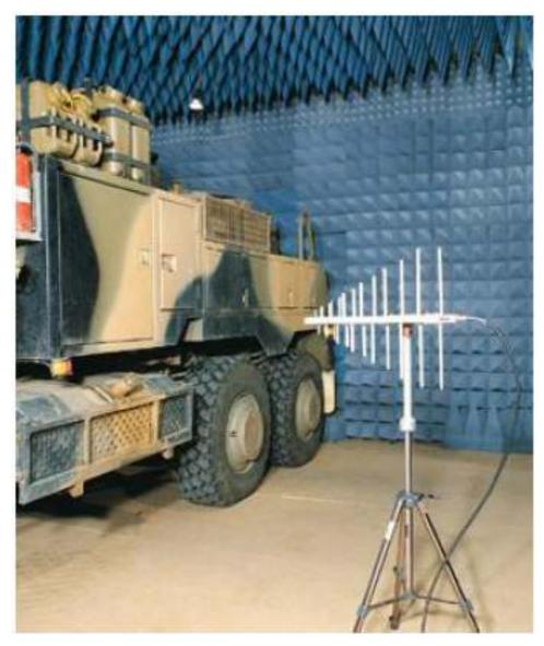
Figure 3.32 Full Anechoic Chamber
