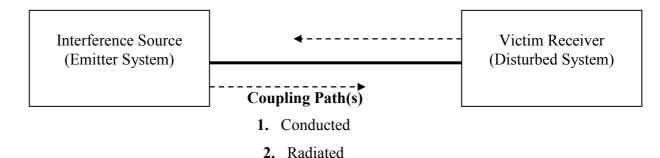
Figure 2.2 Basic EMC model
