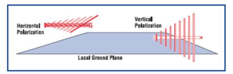
Figure 3.10 Polarization of the antenna
