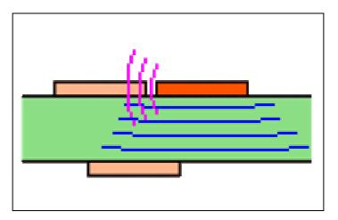
Figure 2.6 Capacitively coupled (electric field)
