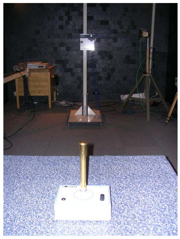
Figure 4.9 Measurement setup of a Field Reference Source in Semi Anechoic Chamber
