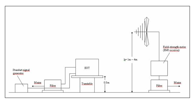
Figure 3.3 Radiated Emission Test Setup.
