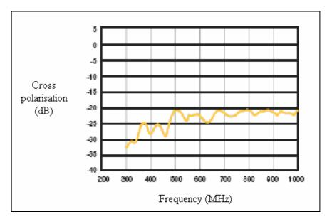
Figure 3.29 CBL 6112 cross polarisation (dB)
