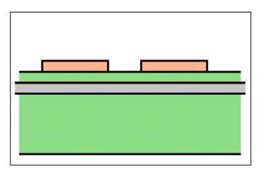
Figure 2.9 Microstrip Transmission Line Characteristic. Impedance affected by Groundplane proximity: Z = Low
