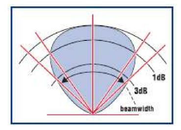
Figure 3.9 Beamwidth of the antenna pattern
