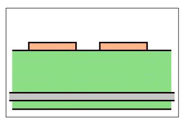
Figure 2.8 Microstrip Transmission Line Characteristic. Impedance affected by Groundplane proximity: Z = High
