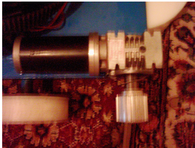
Figure 1.3 Motor, gearbox and trigger gear of the vehicle.
