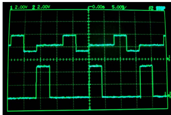
Figure 4.6 Oscilloscope output of the ultrasonic sensors
