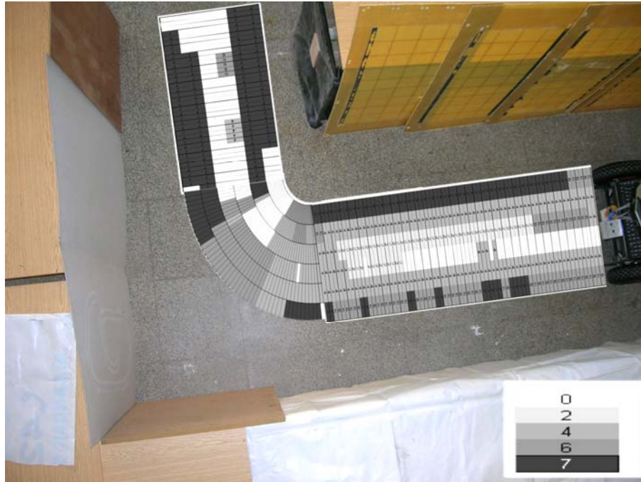
Figure 4.19. Unprocessed signals from ultrasonic sensors which are taken during movement of the mobile robot in a corridor.
