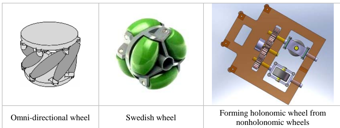
Figure 3.1 Some holonomic wheels and systems. Holonomic wheels are wheels with two degrees of freedom. They are also known as omni-directional wheels or omni-wheels.
