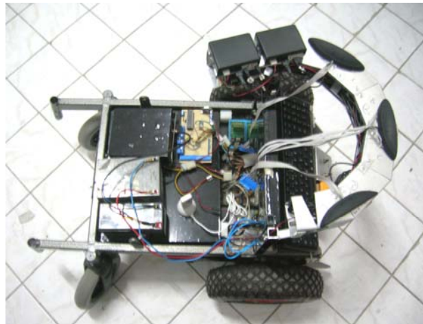
Figure 4.8 Installation of the ultrasonic sensors on real model.
