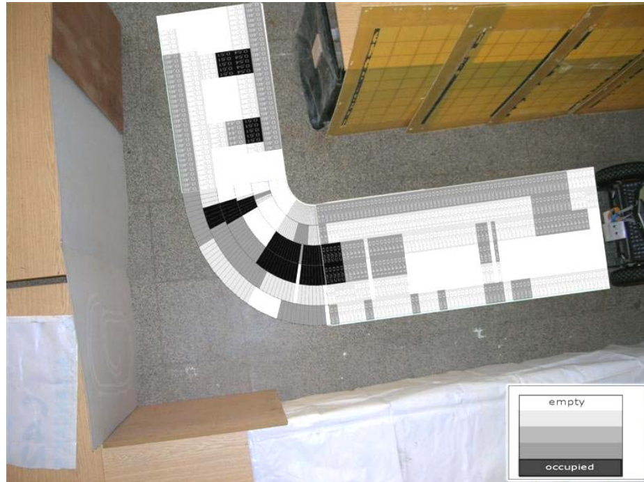
Figure 4.20. Processed signals using DS Theory from ultrasonic sensors which are taken during movement of the mobile robot in a corridor.
