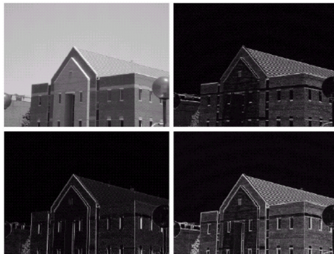
Figure 3.27 a) Original image, b) |G_x| , component of the gradient in the x-direction, c) |G_y| , component in the y direction, d) Gradient image |G_x| + |G_y|
