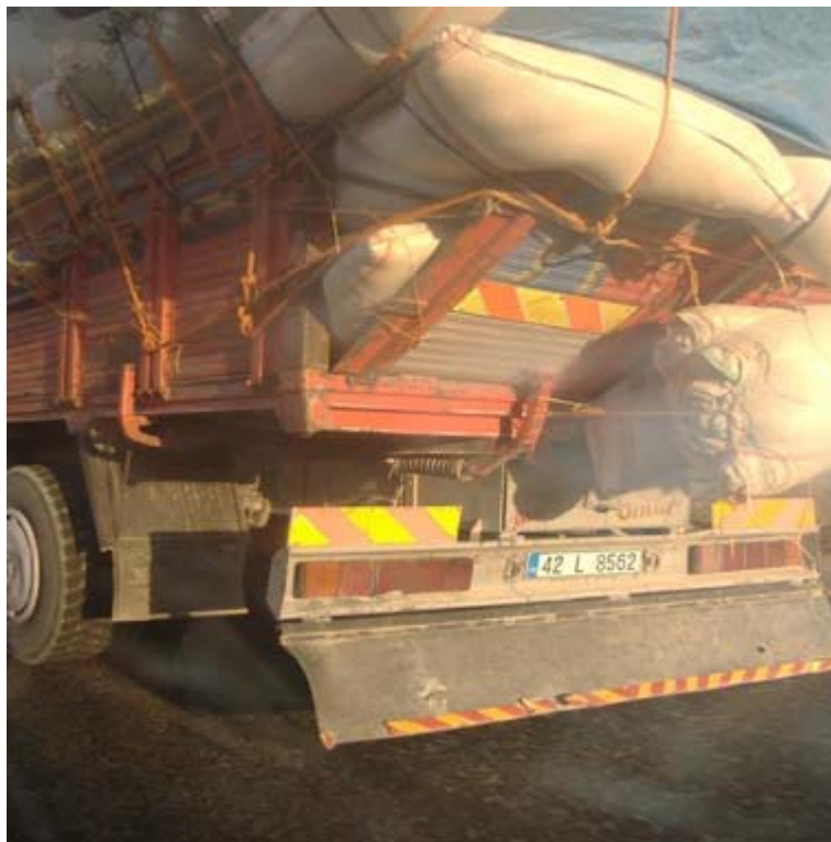
Figure 4.2 This figure shows the possible accident caused by improper placement of materials.
