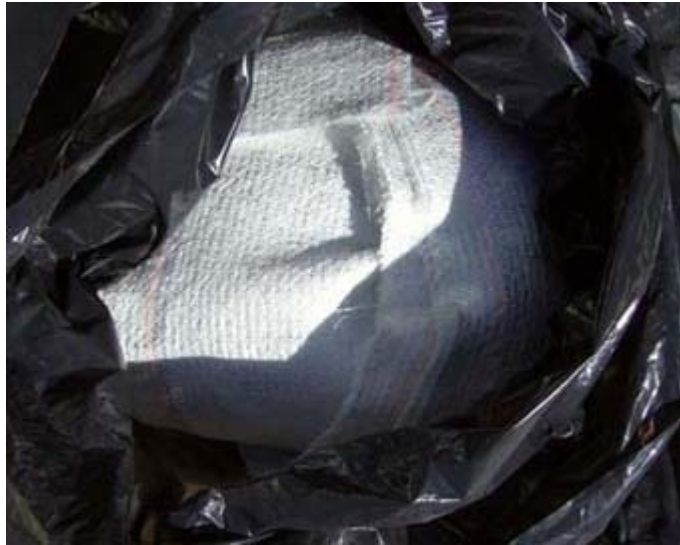
Figure 4.23 Waste glass fabric. It should be collected separately and must not be mixed with other wastes.
