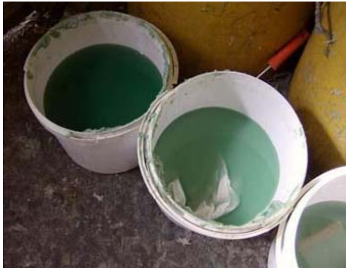
Figure 4.22 Waste organic solvent, hazardous waste. They cannot be drained into sewer or rain drainage system. After being dumped into the described barrels, waste organic solvent barrels should be removed to the place where dye barrels are disposed. After being distilled with the distilling machine, which is purchased in waste minimization plan, waste organic solvent can be used in cleaning especially in maintenance department.
