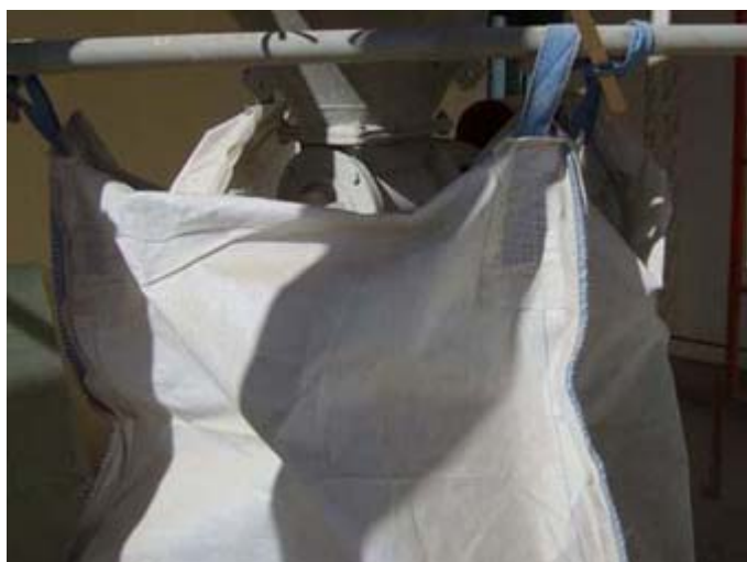
Figure 4.20 Big bags for dust cleaning. The personnel who use this kind of cleaning bag should wear tyvek workwear, dust mask, and gloves.
