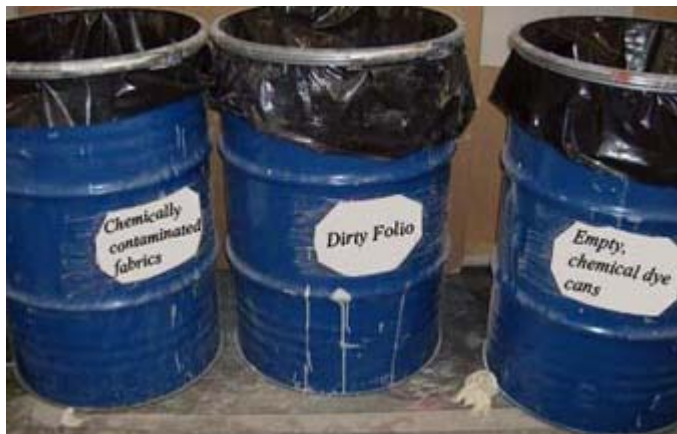
Figure 2.3 This figure is an example for how collection barrels should be ordered in factories.
