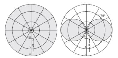
Figure 3.6 Horizontal & vertical signal distribution diagram of RF antenna (Kathrein, 2010).
