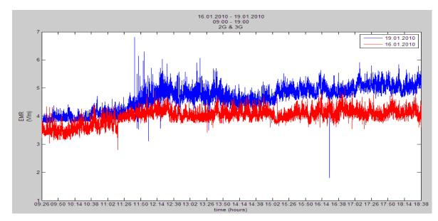
Figure 4.14 Comparison of electric field values recorded at two days
