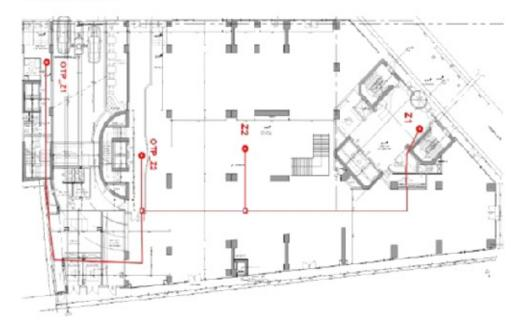
Figure 4.38.b Antenna installation positions: Ground floor (Z1, Z2, OTP\_Z1 and OTP\_Z2)
