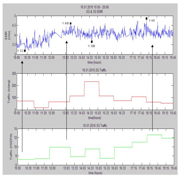
I. Second sector of the base station that operates at dual band for 2G&3G:
