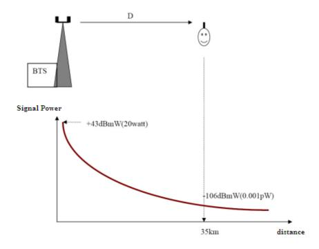
Figure 3.7 Relation between power and distance for GSM (Can, 2006)
