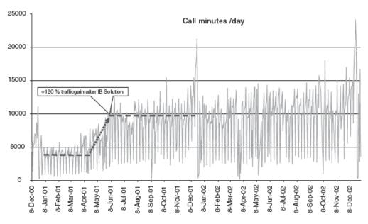
Figure 4.3 The traffic after implementing in-building system in the area covered by macro sites at first (Tolstrup, 2008).
