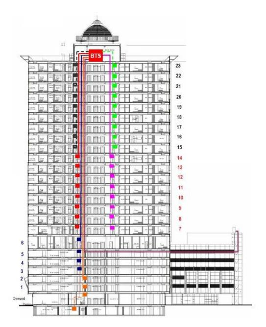
Figure 4.37 In-Building system design of a 23 floored plaza
