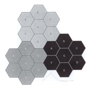
Figure 3.1 GSM cell structure (Tolstrup, 2008)
