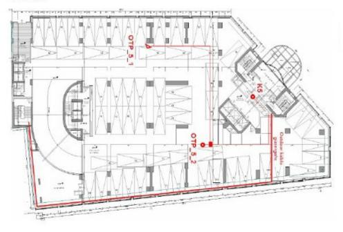
Figure 4.38.d Antenna installation positions: Floor 5 (K5, OTP\_5\_1, and OTP\_5\_2)
