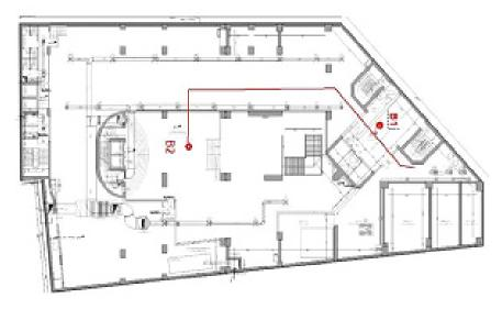
Figure 4.38.a Antenna installation positions: Basement (B1 and B2)
