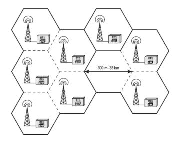
Figure 3.3 BTS distribution in GSM network (Tolstrup, 2008)
