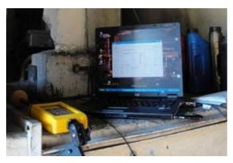
Figure 4.9 EMR-300 connected to PC
