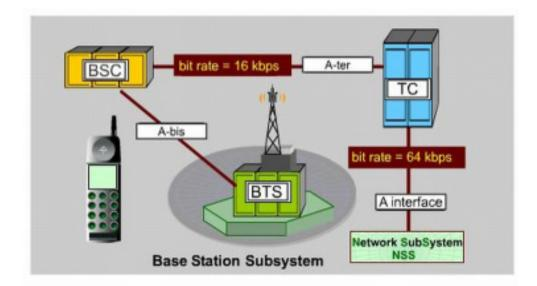
Figure 1.1 Technical block diagram of GSM communication architecture (Heine, 1999).
