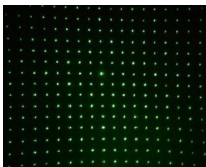
(g) Green light laser beam with matrix pattern
