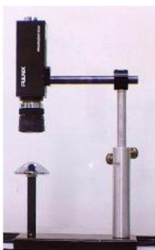
(a) A hyperbolic mirror and perspective camera system
