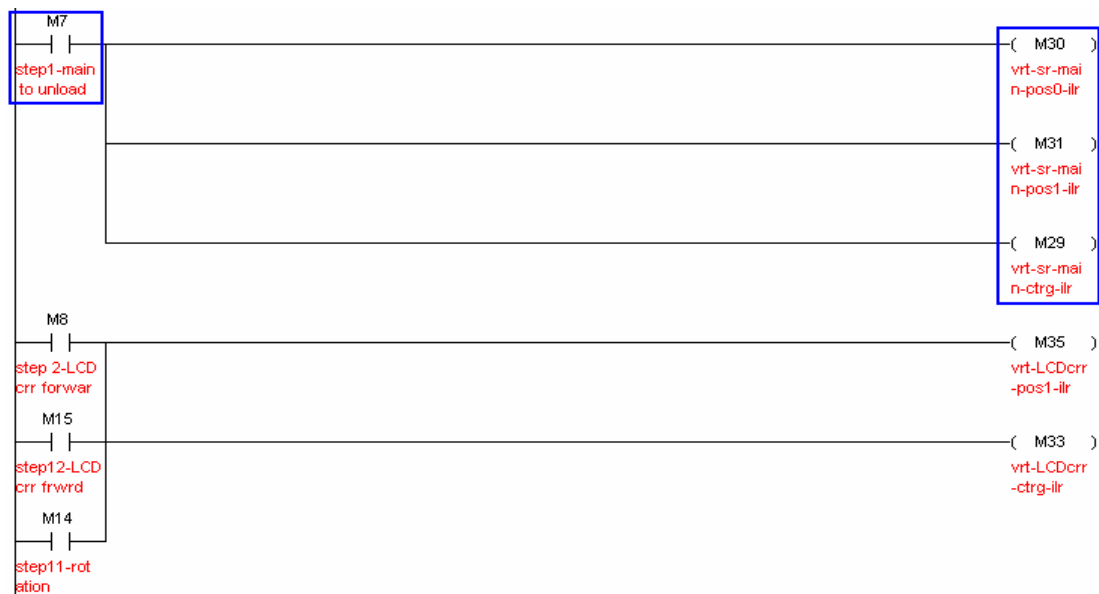
Figure 3.39 Composing the virtual outputs from automatic steps
