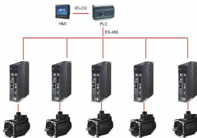
Figure 3.14 Control system of JI silicone dispenser machine
