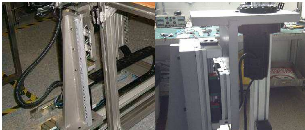
Figure 2.20 Iron support blocks on linear mechanisms
