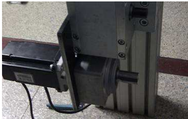
Figure 2.19 Reducer in main carrier mechanism
