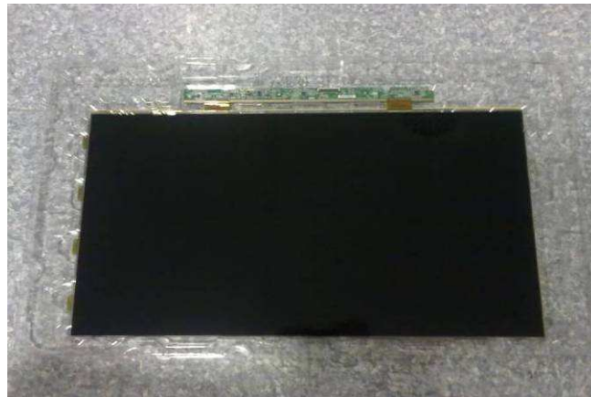
Figure 1.2 An example view of LCD module
