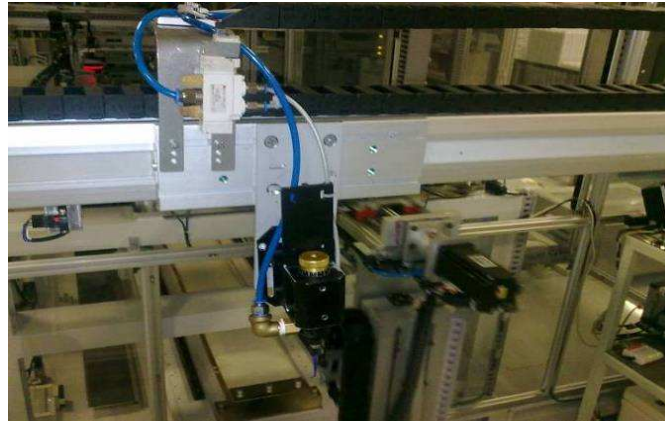
Figure 2.24 Connection between pneumatic valve and silicone injector
