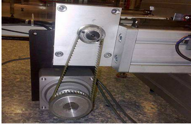
Figure 2.31 Motor connection of main carrier mechanism
