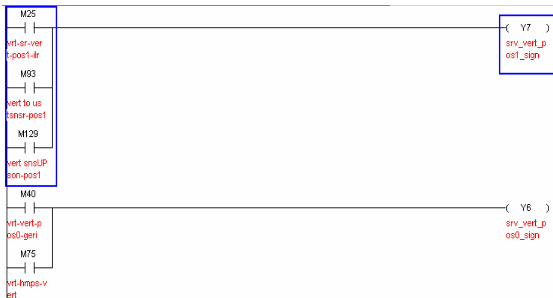
Figure 3.40 Composing of plc outputs with virtual outputs and manual commands
