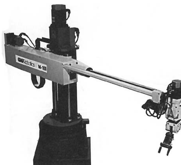
Figure 2.3 A cylindrical robot produced by Seiko Company. (Akdağ, 2008)
