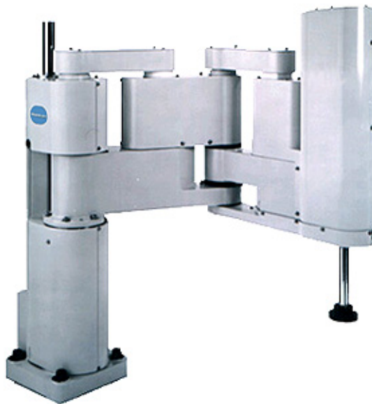
Figure 1.8 Sankyo and IBM, introduced SCARA (Selective Compliant Articulated Robot Arm). (Akdağ, 2008)
