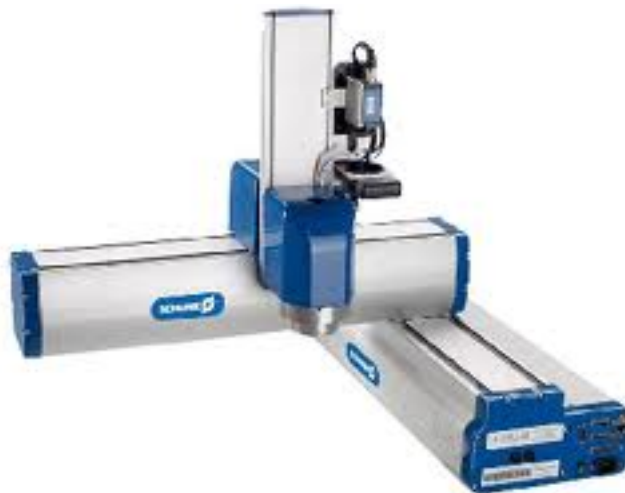
Figure 2.2 Cartesian robot produced by Seiko Company. (Akdağ, 2008)
