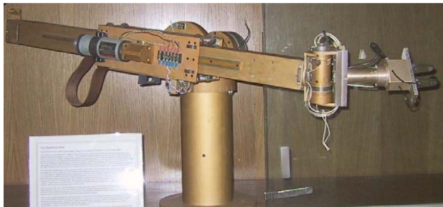
Figure 1.4 Stanford manipulator (Victor Scheinman). (Akdağ, 2008)
