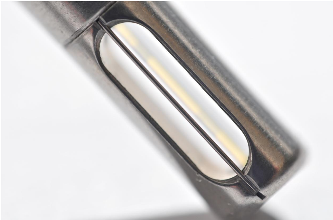
Figure 3.1 a velocity and temperature measurement probe.
