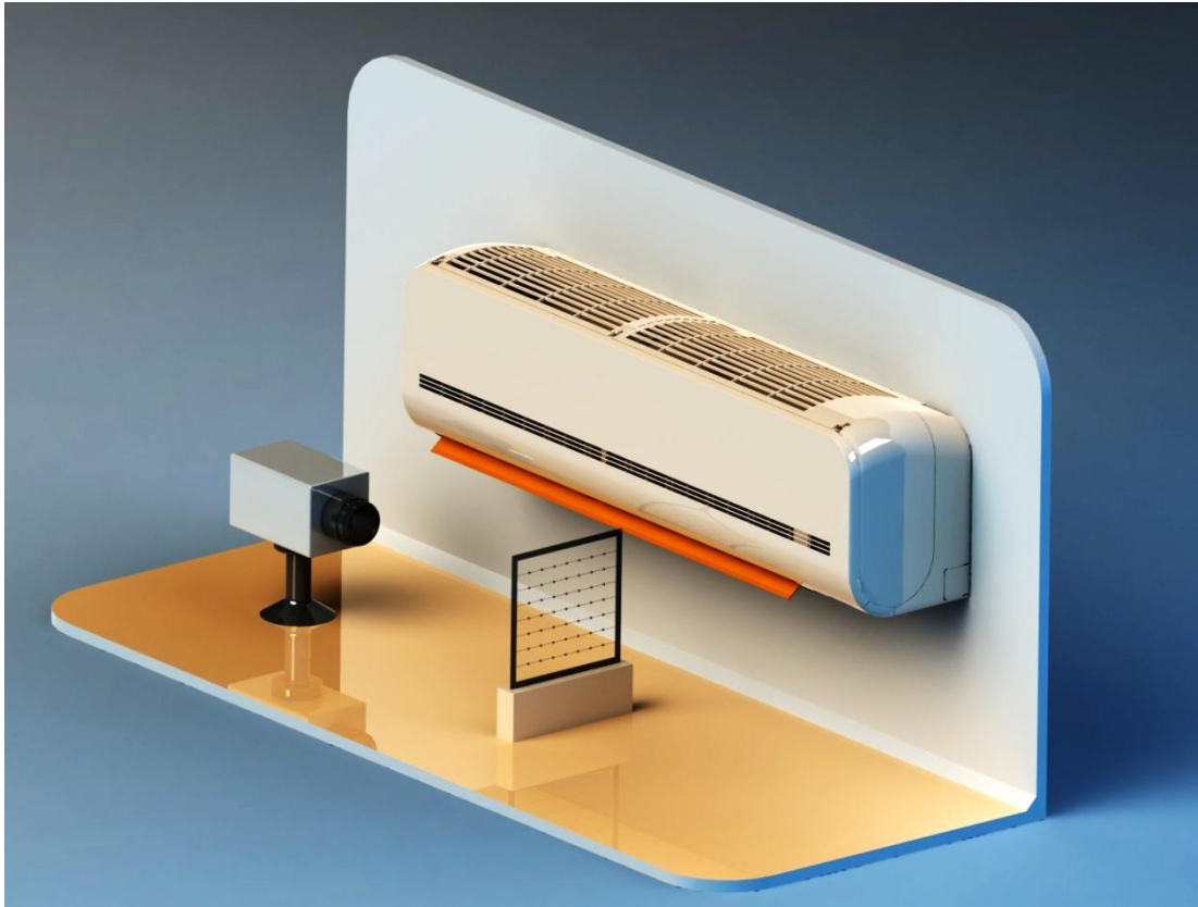
Figure 3.95 the 3d model of MIT measurement at the outflow section of a SAC.
