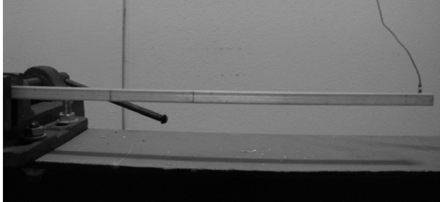
Figure C.1 Cantilever beam used in experiment.
