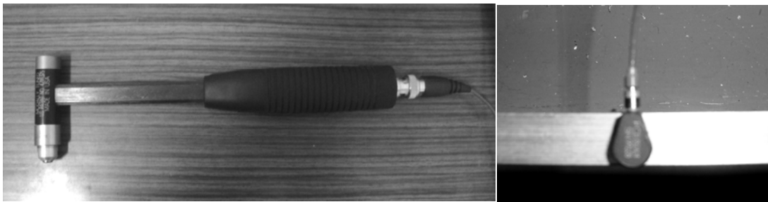
Figure C.2 Impact hammer and miniature accelerometer.
