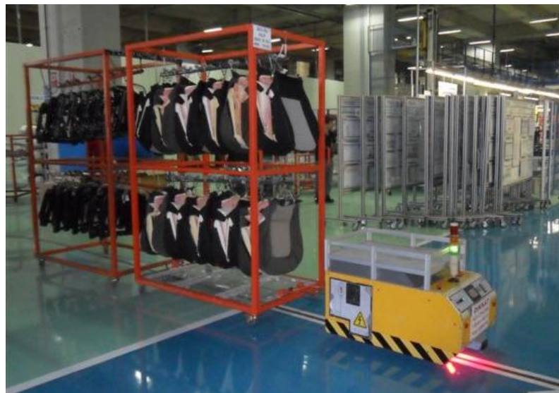
Figure 4.7 The transportation vehicle moves on magnetic tapes.
