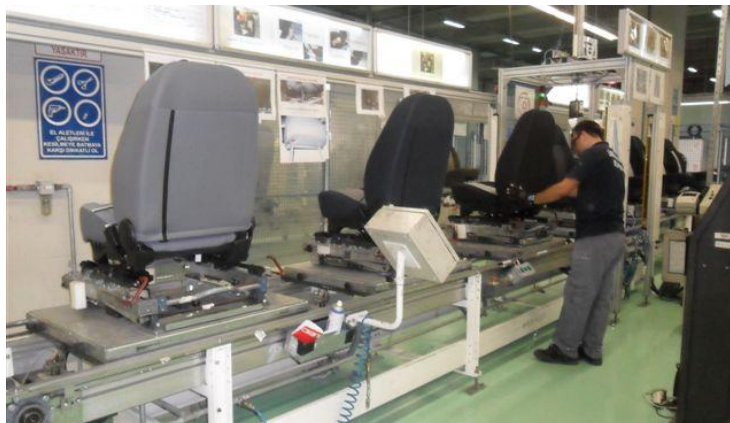
Figure 4.4 Final control station.
