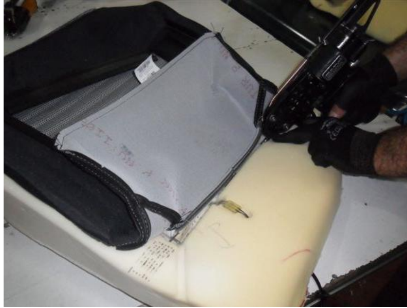
Figure 4.6 The supplementary units that is hooked slipcover to foam.
