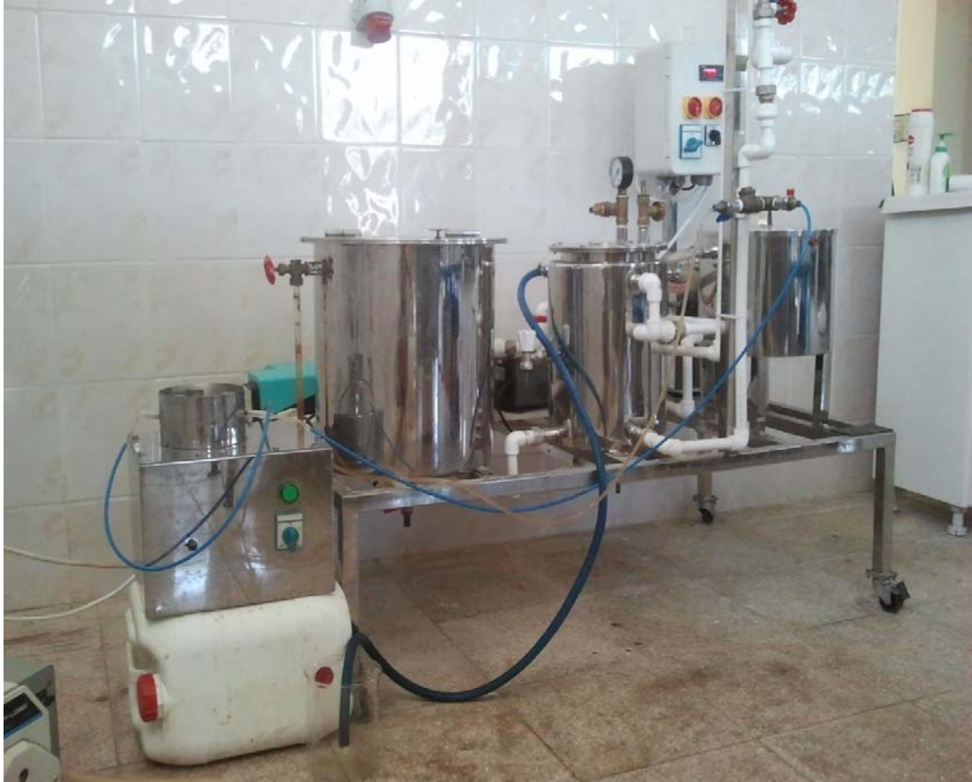
Figure 4.3 The view of the anaerobic model reactor system used in experimental studies.
