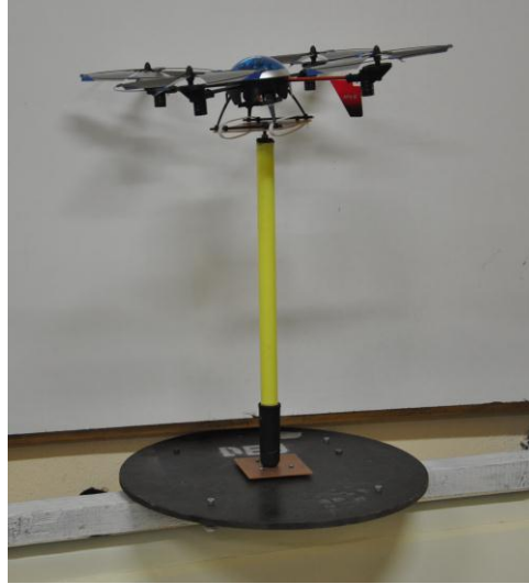
Figure 3.5 Designed testbed lateral view.
