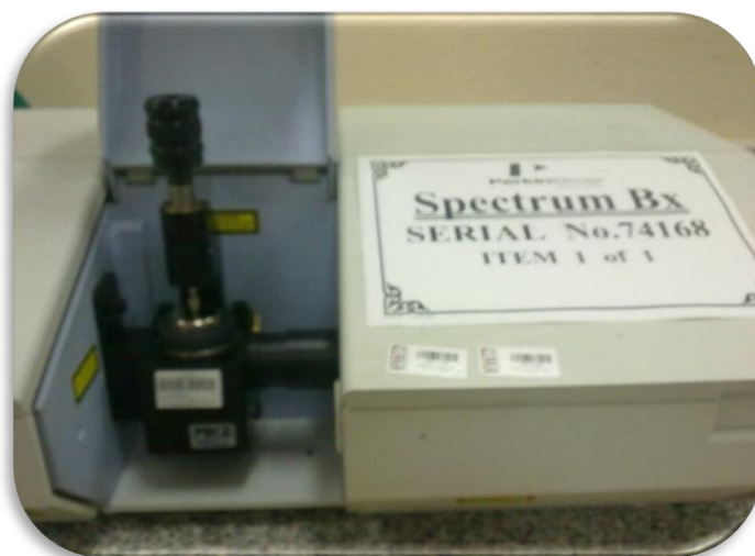
Figure 3.16 Schematic illustration of FTIR system having ATR apparatus (Electronic Materials Lab., DEU).
