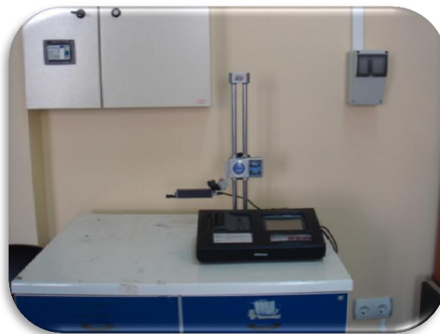
Figure 3.22 Mitutoyo SJ-301 surface (Tribology Lab., DEU)
