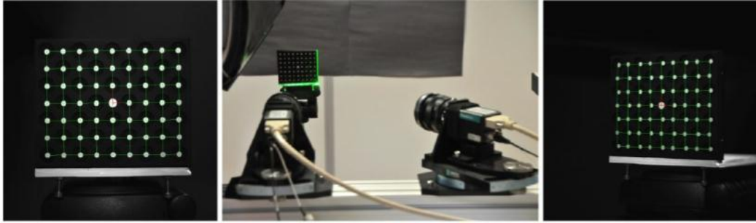
Figure 4.5 Calibration target and cameras (Özer, 2011).
