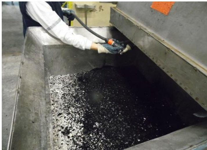
Figure 4.13 Cleaning of the kibble with water jet
