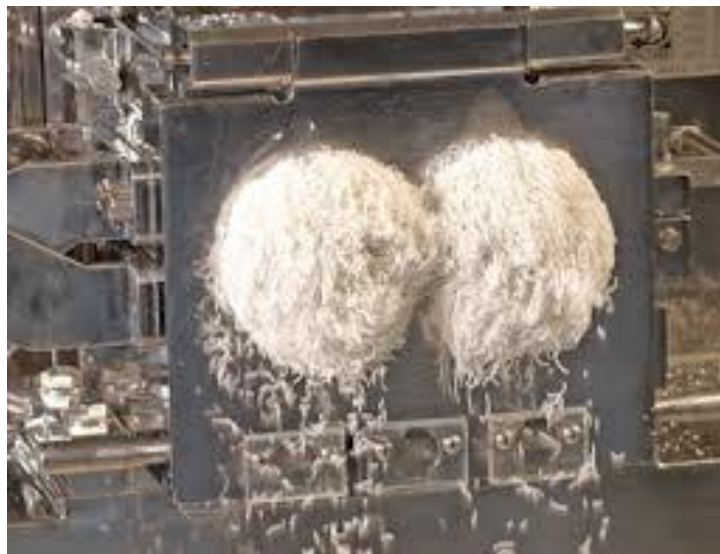
Figure 4.9 Photograph of extruder cleaning with resin and PVC
