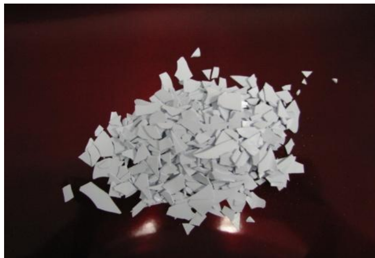
Figure 4.5 Photograph of powder coating chips
