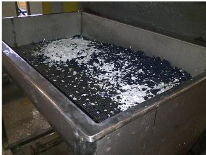
Figure 4.14 Cleaning resins collected in the new container (tank)
