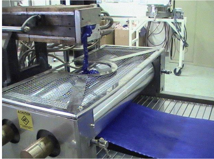
Figure 4.4 Photograph of extruder cooling band
