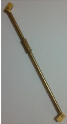
Figure 3.7 A view of the diagonal which was used at first storey to represent undamaged specimen case.
