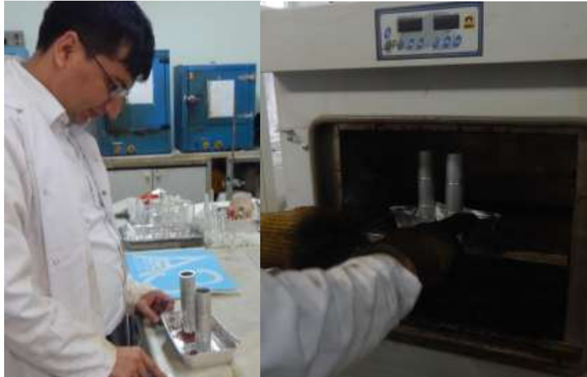
Figure 7.5 General view of the filled and sealed tube for the storage stability test
