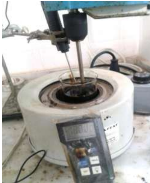
Figure 7.16 Production of polymer modified bitumen
