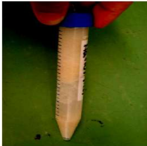
Figure 1.6 Phase separation of a salt hydrates (Streicher, Cabeza and Heinz, 2005)
