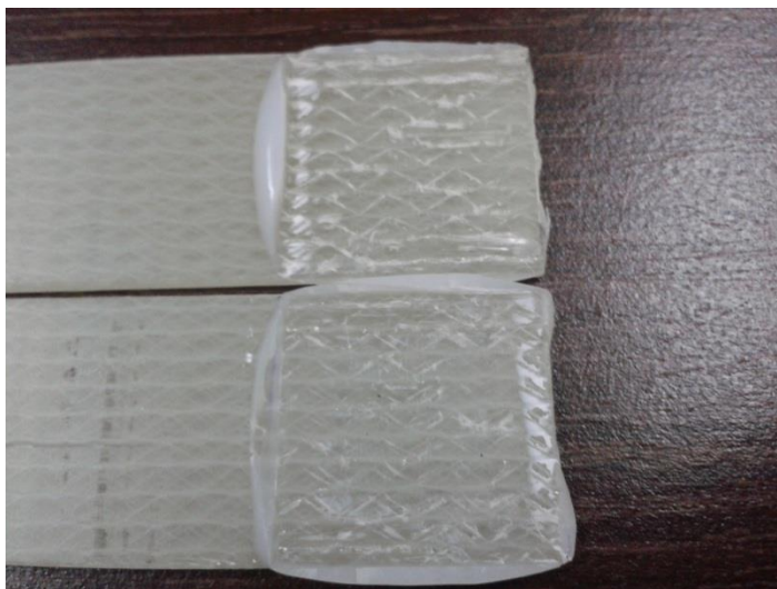
Figure 4.47 The test specimen, Original surface and L/L1= 2,5 (Failure mode: Composite adherends interlaminar fracture and Adhesive bondline fracture)
