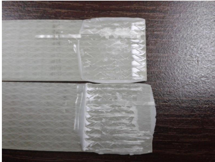
Figure 4.44 The test specimen, sandblasted and L/L1= 2,5 (Failure mode: Composite adherends interlaminar fracture)
