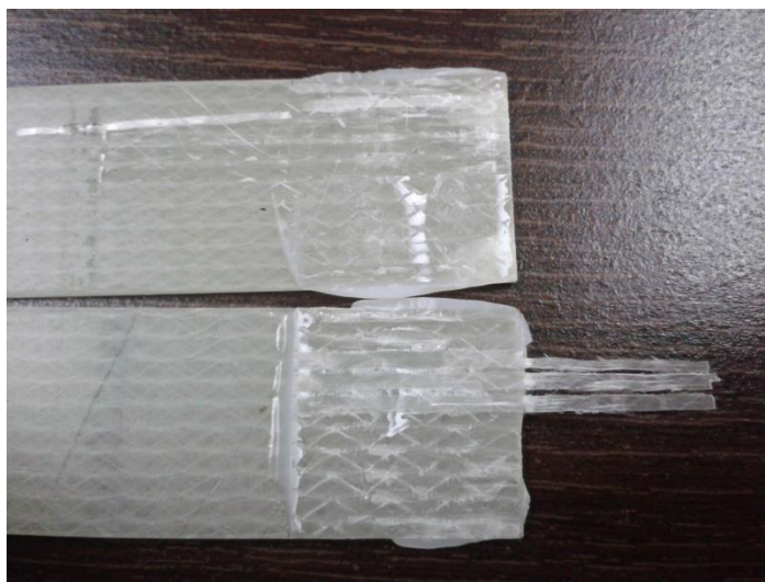
Figure 4.45 The test specimen, Orjinal surface and L/L1= 1,5 (Failure mode: Composite adherends interlaminar fracture)
