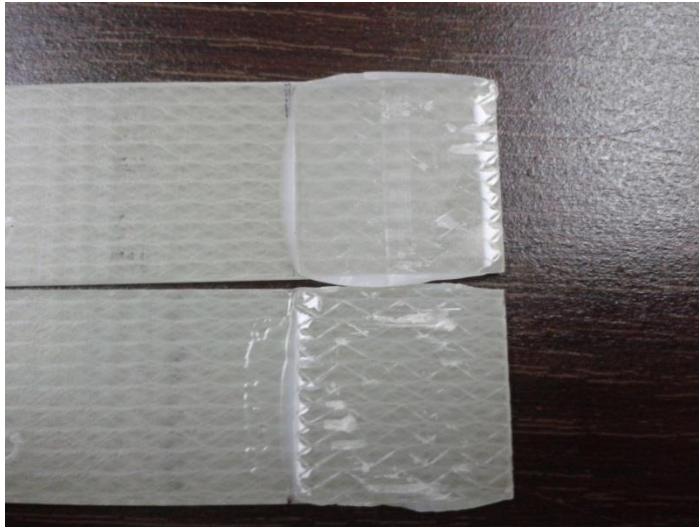
Figure 4.46 The test specimen, Original surface and L/L1= 2 (Failure mode: Composite adherends interlaminar fracture and Adhesive bondline fracture)
