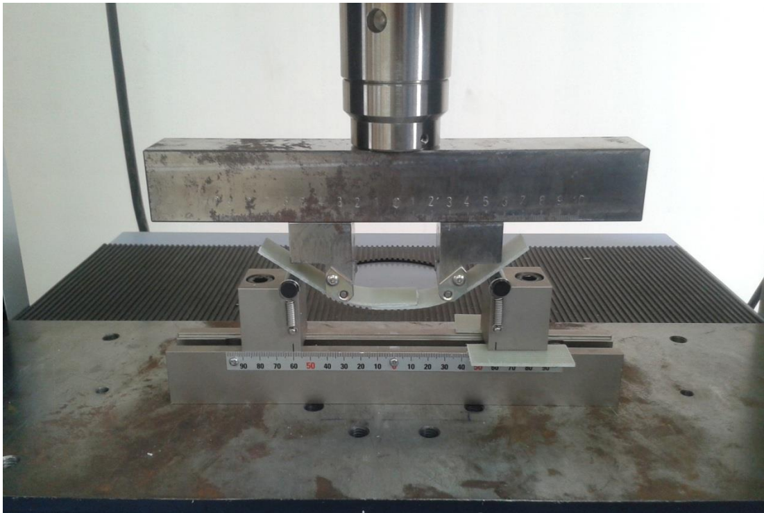
Figure 3.11 Four point bending test apparatus and specimen positioning
