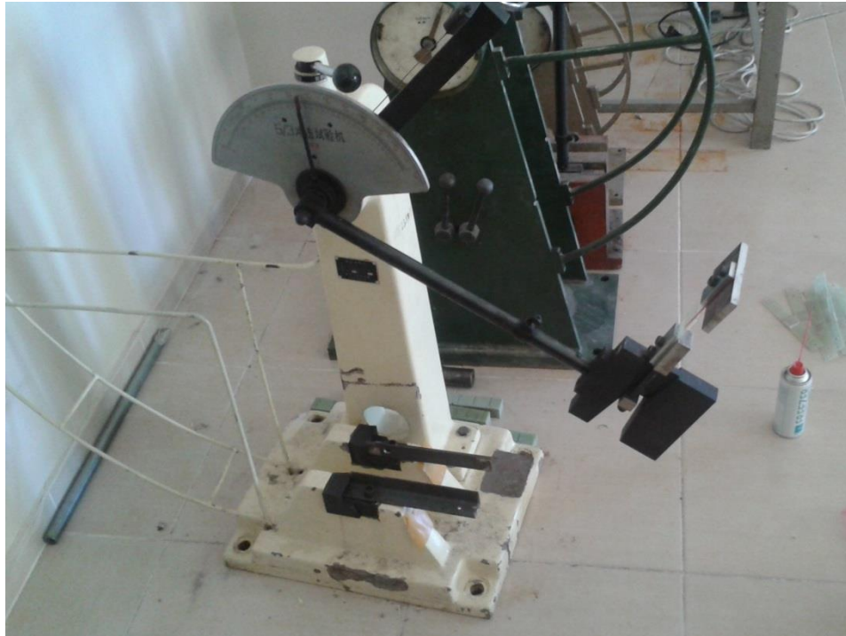
Figure 3.7 Impact test device with the specimen installed
