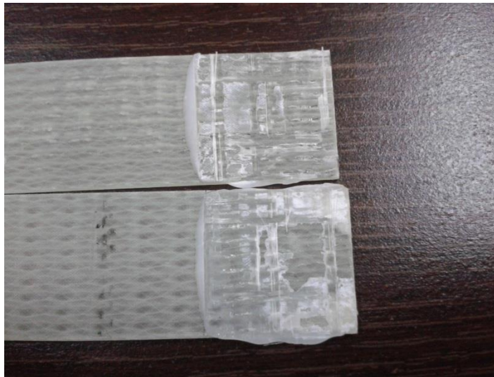
Figure 4.43 The test specimen, sandblasted and L/L1= 2 (Failure mode: Composite adherends interlaminar fracture and Adhesive bondline fracture)
