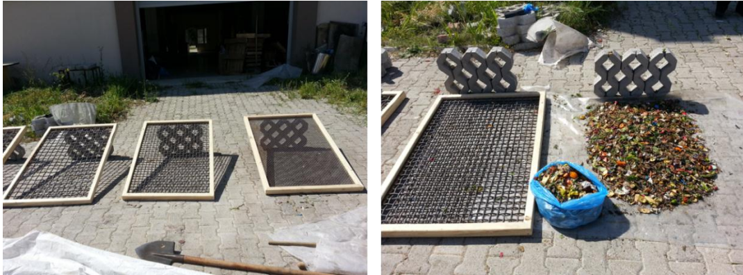
Figure 3.4 The screens and the example of the undersized solid wastes
